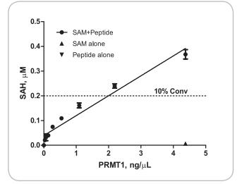
Figure 4. Linear relationship between PRMT1 concentration and SAH formation. The polarization values were converted into SAH (product formed) using a standard curve set up under similar conditions.
