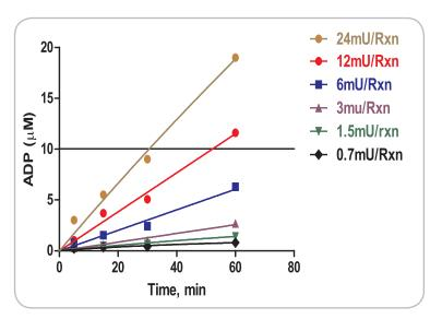
Figure 1. Initial rates of PKA enzyme in triplicates of 20  $\mu$ L reactions containing varying amounts of PKA, 100  $\mu$ M ATP and 100  $\mu$ M Kemptide showing the amount of product formed with time.
