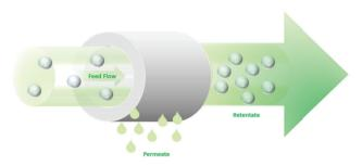
Our TFF-Easy is a filter cartridge containing hollow fibers made of polysulfone suitable for the concentration and the removal of small proteins and molecules from diluted matrices (cell conditioned media, urine, etc..), prior to the EV purification.
