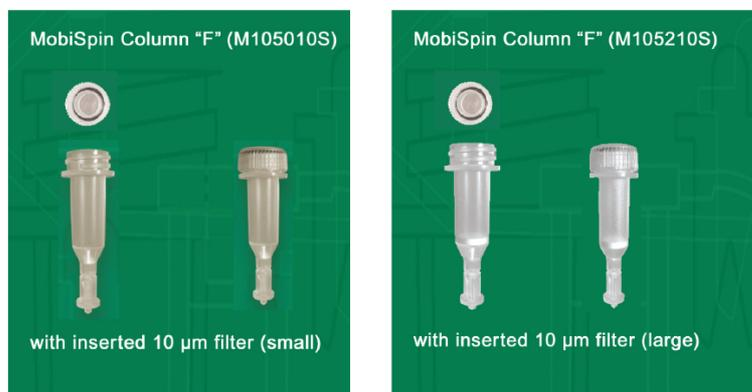
The MobiSpin Column "F" comes with inserted filter of 10 µm pore size, screw cap and snap-off plug. It can be used without matrix (e.g. to extract trypsinated proteins out of a gel slice for Mass Spec analysis) or filled with a matrix of your choice.
