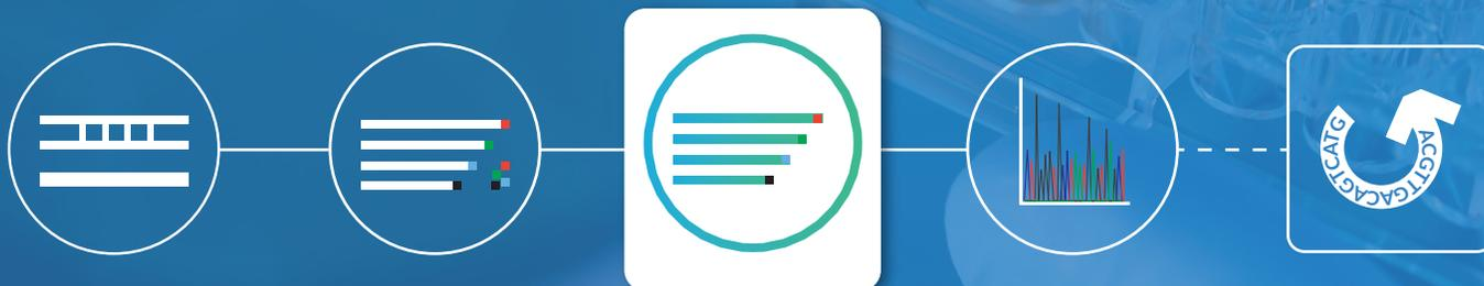
It is essential to remove the contaminants, especially the unincorporated ddNTP dyes, from the completed sequencing reaction. Failure to remove these contaminants results in signal reduction and interference of peak separation and reading.
